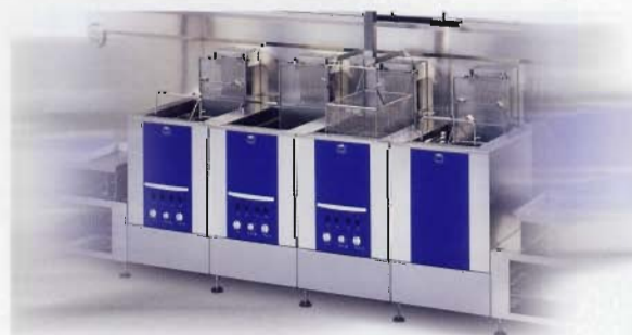
Automated cleaning line, 4 chambers, with dryer and agitation
